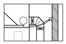
**NOTE:** Screws to attach the cable bracket have not been provided because of the variation of wall surfaces. Select the correct type of fasteners for your type of wall construction.
